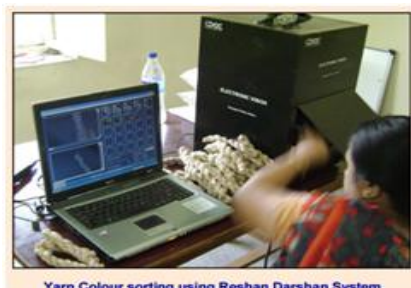
Yarn Colour sorting using Resham Darshan System
